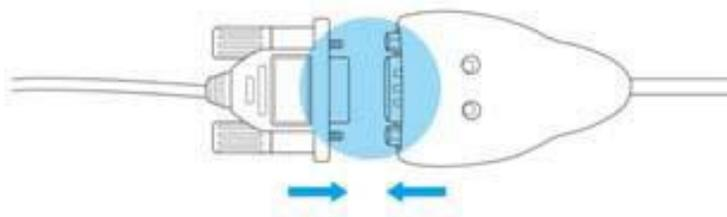
\*If the gender of the serial port of your computer or laptop is not correct, you may need to use a Serial to USB Converter or Serial Gender Converter.
