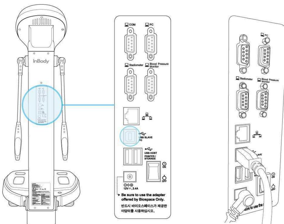
2) Plug the USB host end of the USB cable into the USB port of your computer or laptop.
